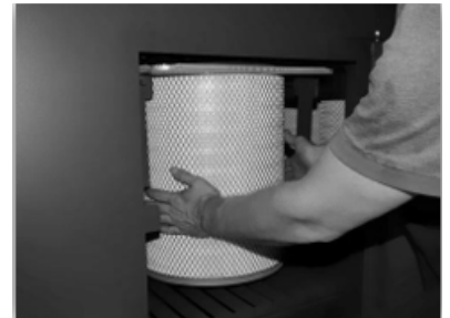
3. Slide filter cartridge(s) out
