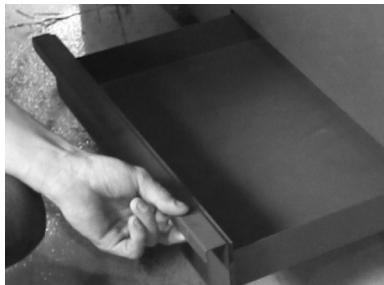
5. Open dust drawer and remove material.
