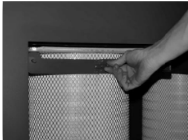
2. Unhook barrel bolt latch.
