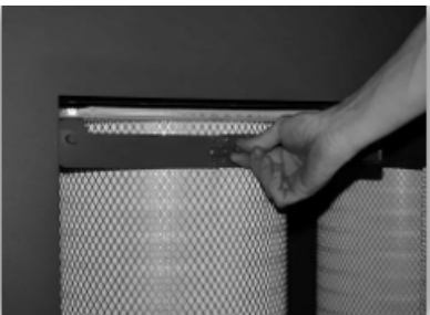
7. Hook barrel bolt latch.
